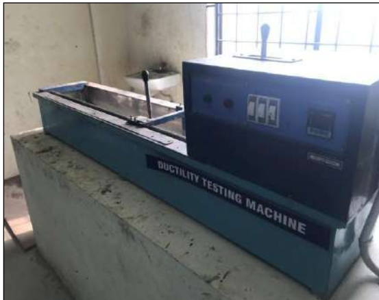
Ductility testing Machine
