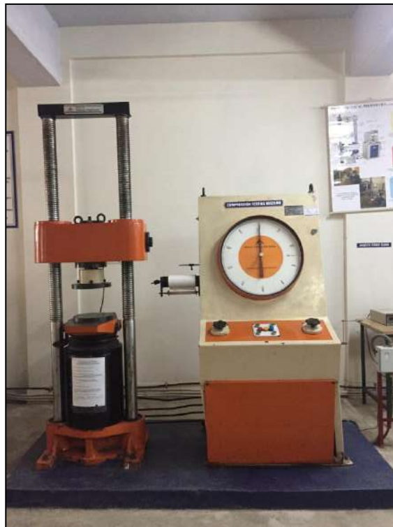
Universal testing machine with double shear chuck
