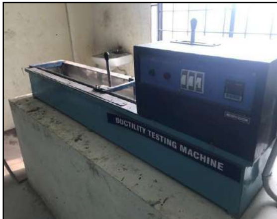
Ductility testing Machine
