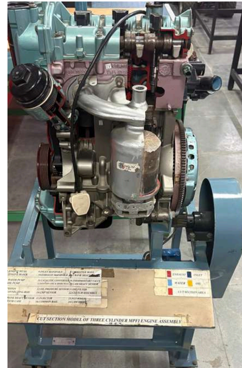
CUT SECTION MODEL OF THREE CYLINDER MPFI ENGINE ASSEMBLY
